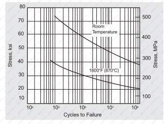
Figure 3. Rotating-beam fatigue strength of solution-annealed INCONEL alloy 617.
